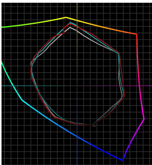
Roland SG2-540 color gamut compared against Adobe RGB(1998) color space (multi-color graph)
